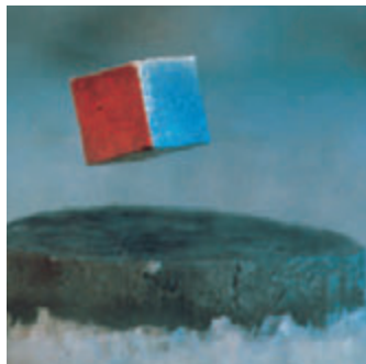
A small permanent magnet levitated above a disk of the superconductor \text{YBa}_2\text{Cu}_3\text{O}_7 , which is in liquid nitrogen at 77 K.
