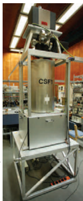
Figure 1.1 (a) The National Standard Kilogram No. 20, an accurate copy of the International Standard Kilogram kept at Sèvres, France, is housed under a double bell jar in a vault at the National Institute of Standards and Technology. (b) A cesium fountain atomic clock. The clock will neither gain nor lose a second in 20 million years.
