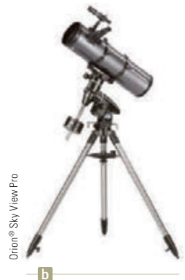
Figure 36.43 (a) A Newtonian-focus reflecting telescope. (b) A reflecting telescope. This type of telescope is shorter than that in Figure 36.42b.
