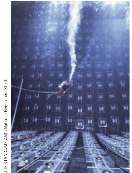
Figure 46.6 (Example 46.2) A diver swims through ultrapure water in the Irvine–Michigan–Brookhaven neutrino detector. This detector holds almost 7 000 metric tons of water and is lined with over 2 000 photomultiplier tubes, many of which are visible in the photograph.
